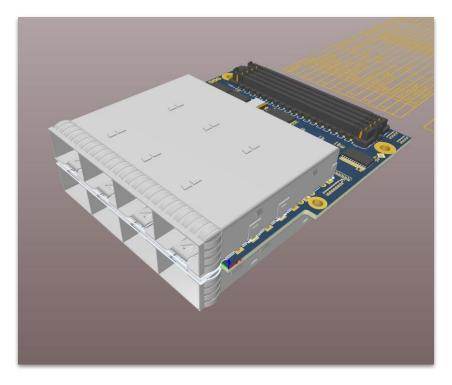
Developed a mezzanine card with 8 SFP+ Channels.
